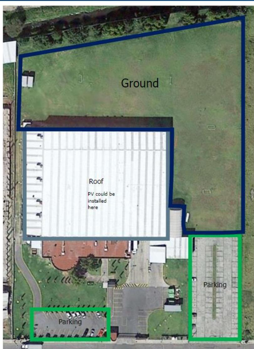
The image to left, provided by ZF, shows the existing ZF facility, pre-expansion. An expansion project is planned for 2023 which will cover the existing ground area with additional building facilities (and thus roof space for PV). The following table estimates the land, roof, and carport areas for PV *after* that expansion.
